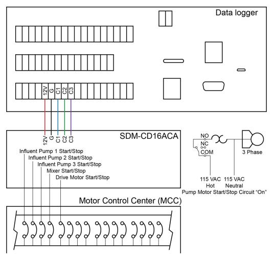
Figure 4-3. SDM-CD16ACA relay outputs to MCC
