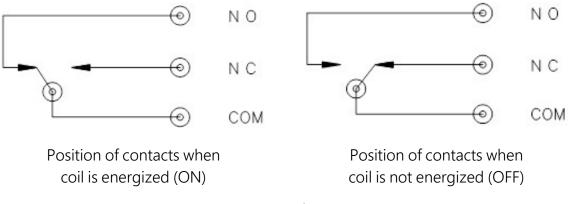
Figure 4-1. Switch operation
